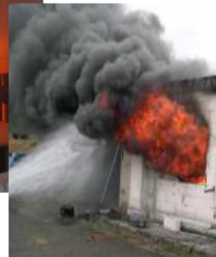
Figure 4. Gas temperatures at the ceiling level. From 4 min (upper photo) onward the temperatures increased fast and the fire developed violently. The flashover situation (lower photo) was reached some 10 min after ignition and the test was interrupted at about 15 min by manual intervention.
